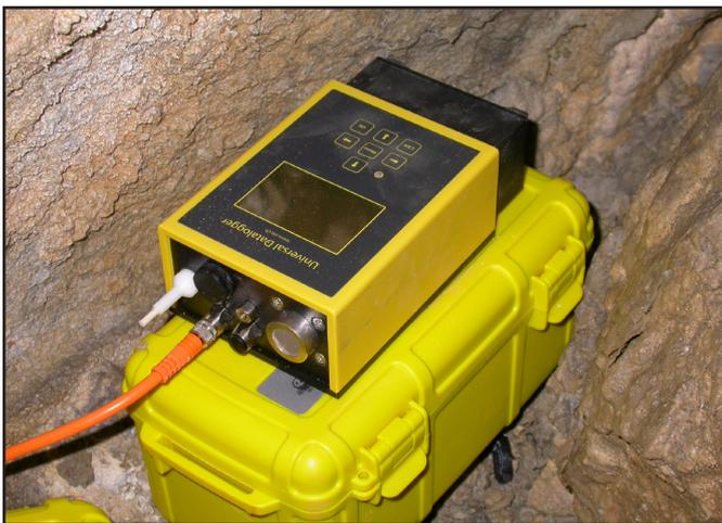
Fig. 1. The CORA device used for monitoring CO<sub>2</sub> concentrations in cave air. The yellow box underneath the device holds eight 1.5 V batteries (D cells).
